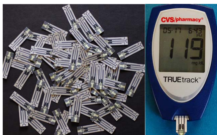
Figure 2.3: Microfabricated paper-based analytical chips and their application in a commercial hand-held glucometer. Figure adapted from [17].
